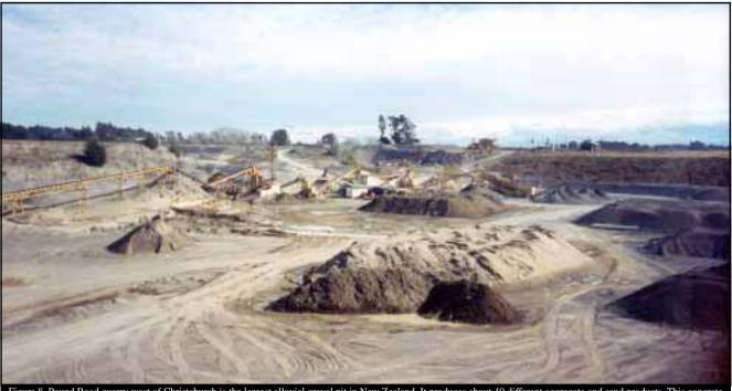
Figure 8. Pound Road quarry west of Christchurch is the largest alluvial gravel pit in New Zealand. It produces about 40 different aggregate and sand products. This concrete aggregate and chip processing plant is one of three plants in the quarry. Photo: Fulton Hogan Ltd.
