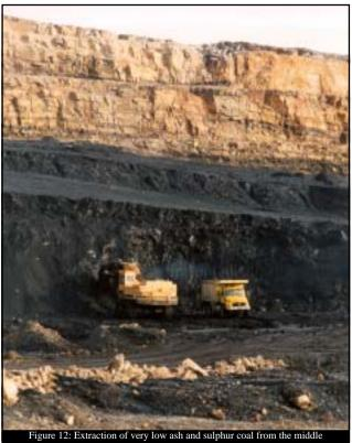
Figure 12: Extraction of very low ash and sulphur coal from the middle of the thick Mangatini Seam in Webb opencast mine at Stockton in the Buller Coalfield (photo: Lloyd Homer).
