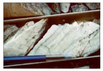
Figure 2: Banded quartz of the Birthday Reef in hole WA11A at Blackwater (Waiuta), drilled by Macraes Mining in late 1996 (Photo: Tony Christie).
