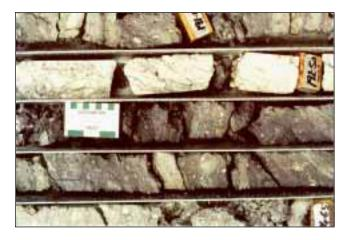
Figure 3: Gold-bearing quartz lode and adjacent clay-rich breccia in drillcore from the Globe-Progress prospect in Reefton (Photo: Tony Christie).
