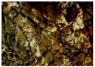
Figure 8: Stockwork quartz veins exposed in the Golden Cross open pit (Photo: Tony Christie).
