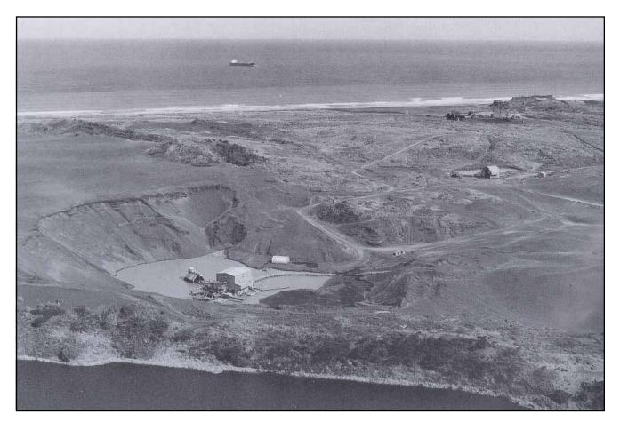
Figure 5: Taharoa ironsand mining operation has a dredge and concentration plant (foreground), dry mining plant, offices, workshops and stockpile (right centre). The Taharoa Maru, 2.5 km offshore, loads ironsand by an undersea pipeline (Photo: BHP New Zealand Steel Ltd).
