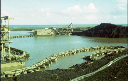
Figure 6: Ironsand dredge and floating concentrating plant at the former Waipipi mine, near Waverley (Photo: Bruce Thompson).
